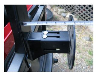
Using the measurement from the step before. Measure from the antenna post to the front side of the wheel hub. Use 2 @ 5/16" x 3/4" carriage bolts, 2 flat washers and 2 locking nuts to tighten the top of the wheel hub down. After the top bolts are tight use 2 @ 5/16" x 3/4" carriage bolts, 2 flat washers and 2 locking nuts to tighten the side of the wheel hub down.
