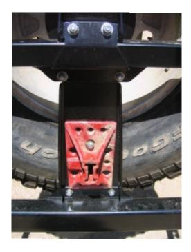
Before installing Hi Lift remove the foot off of the jack. The foot can be bolted in the backside of the antenna post using a 5/16" x 1" carriage bolt with a washer and locking nut.
