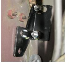
Drill from the cargo area thru the tub using a 7/16" drill bit.
