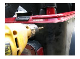
Remove the upper hinge arm from the tire carrier.
