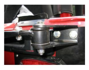
Remove the outside roll cage bolt.
