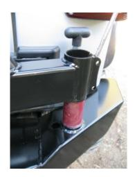
Lube the spindle on the bumper with auto or marine grease
